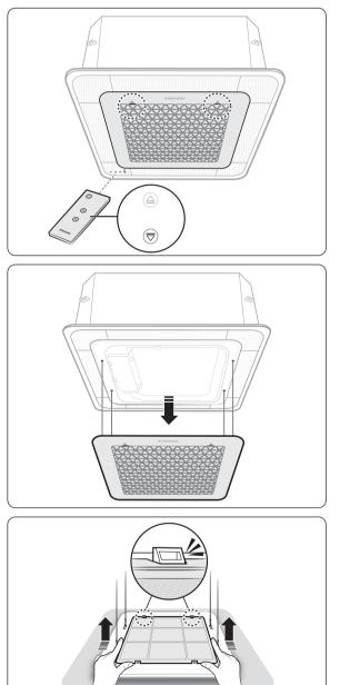
Press the [Grille Down] button to move down the grille.
