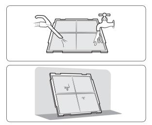
Clean the air filter with a vacuum cleaner or soft brush. If dust is too heavy, then rinse it with running water and dry it in a ventilated area.
