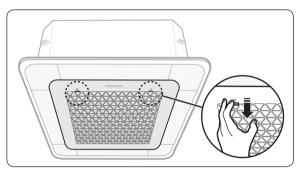
Push down the hooks at each side of the front grille to open the grille.
