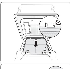
Fit the air filter on the front grille.
