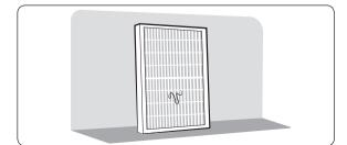
Clean the filter as follows: Immerse it for about 30 minutes in lukewarm water with neutral detergent diluted and shake it up/down several times.
