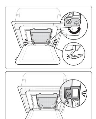
Turn the latches after removing the safety hooks.
