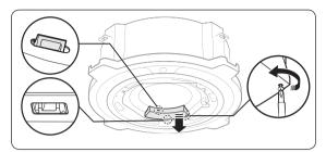
4 Fix the lift kit to the indoor unit by pressing the hook, and then tighten the screws.
