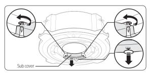
6 Connect the earth, power and signal cables, and then fix the wiring as shown in the figure. Next, attach the electrical system unit cover and then the sub cover.
